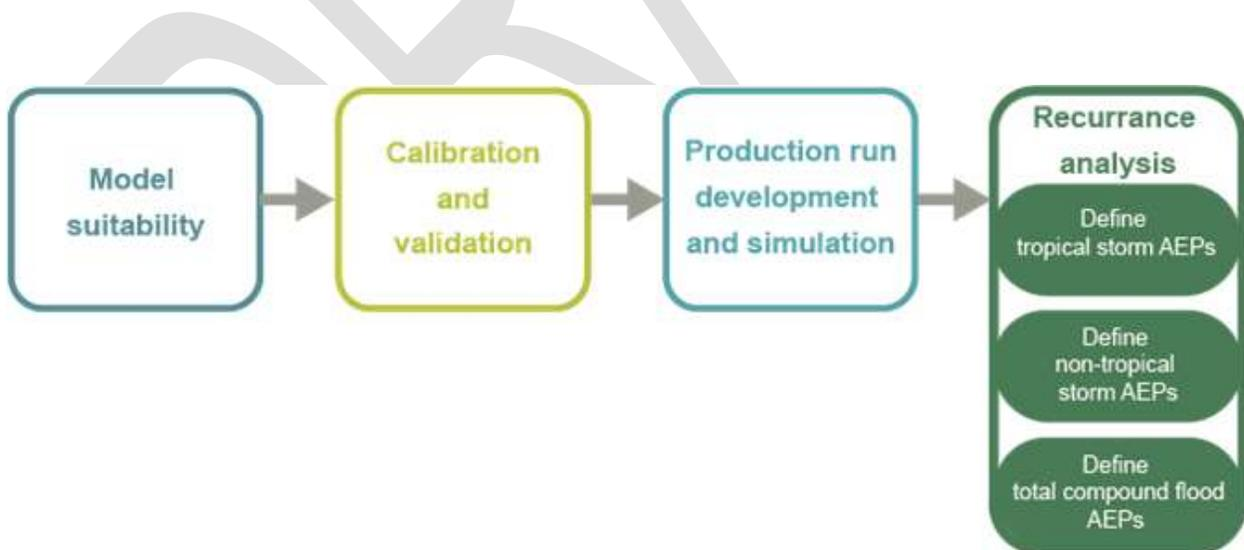
Figure 17: Diagram of elements of recurrence analysis component of the study methodology.
