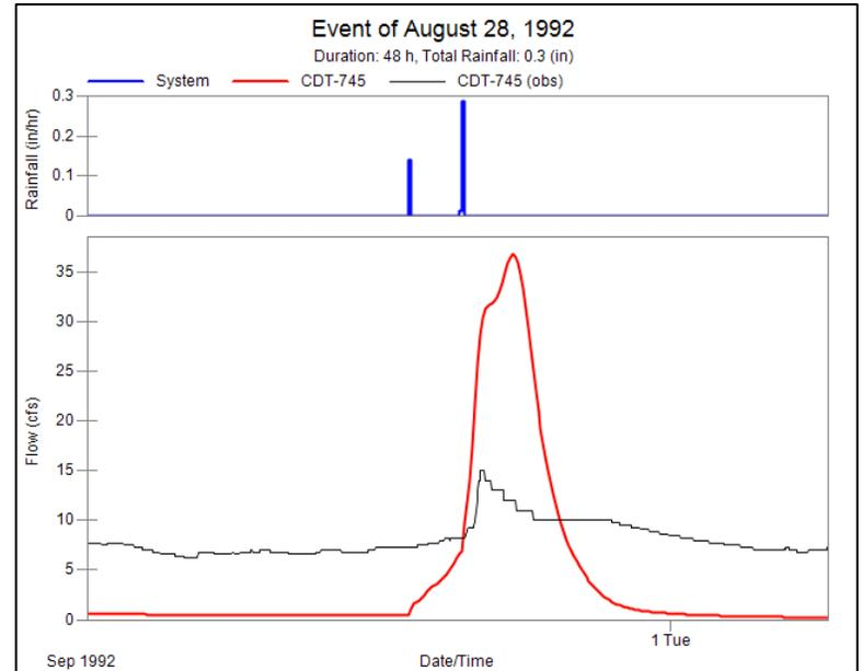
**Figure 4-9: Modeled vs Observed hydrographs for four events at Falling Creek Gage**
