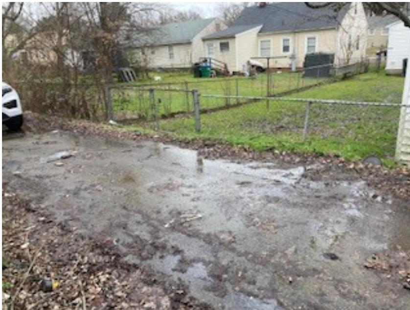
Figure 4: Photo of flooding at location 2. Ponding is visible and seen to be flowing into the backyard of residential property 1413 Willis Street.
